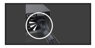
Leave enough 12VHPWR cable length (around 35mm), then do cable management. The connectors should click to lock in.
