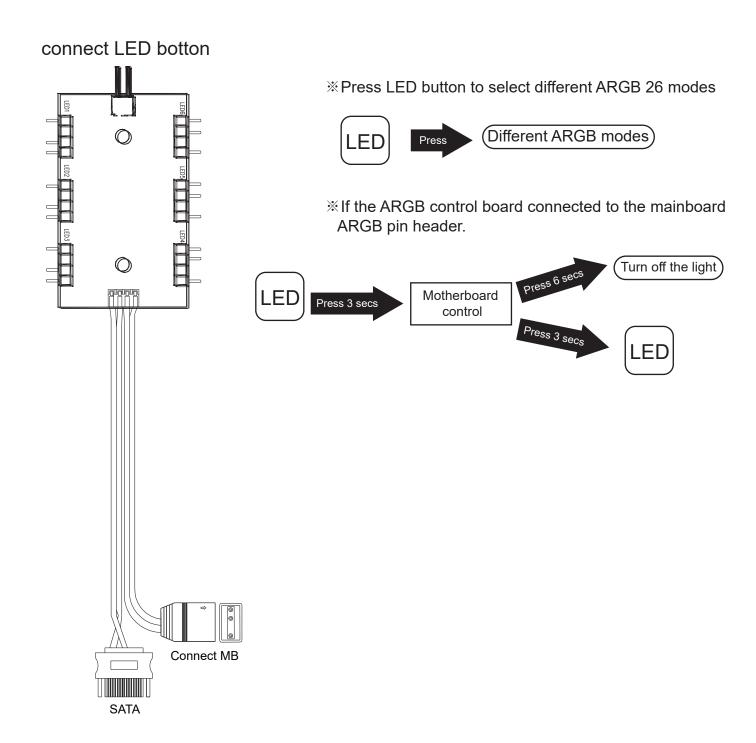
If the ARGB control board connected to the mainboard ARGB pin header,
