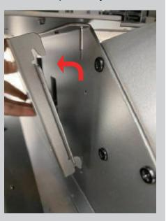
Disk Drive Mounts on both sides: Two 2.5" drives or one 3.5" drive
