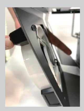
•When installing fans only: Use nuts on the rear of the screw to affix the fan onto the chassis as shown.
