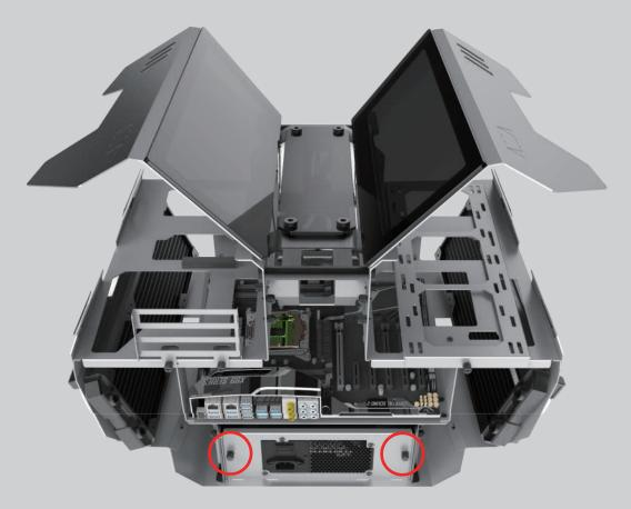
Loosen the hand screws to remove the power supply bracket. Attach the power supply to the bracket before placing it back in.
