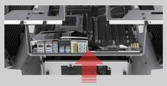
(3) Screw the motherboard onto the tray through the chassis.
