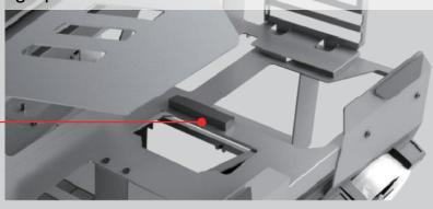
PCI-e cable installation: Plug the cable onto the motherboard by passing the cable through the hole as shown
