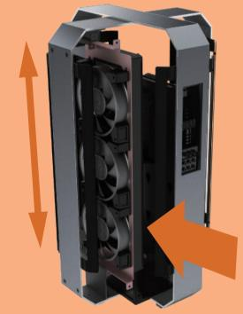
Please install the CPU bracket and radiator pump into the motherboard before pushing the cooler into the chassis
