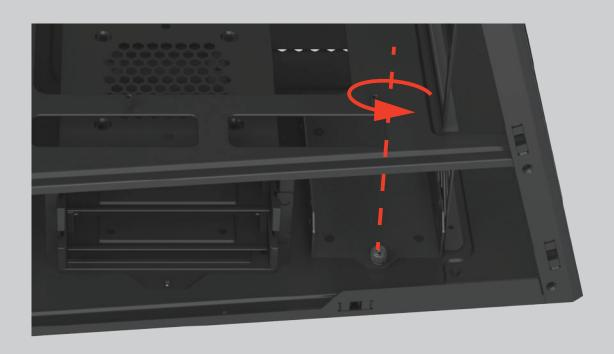
If you want to install SSD, unscrew the screw and remove the SSD tray
