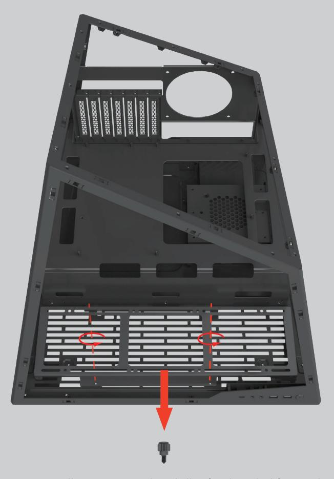
Unscrew the screws and push the fan bracket forward
