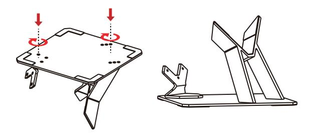
2. Then attach the base to the rear of the case by flipping the case onto its front
