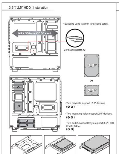
Secure 2.5" SSD / HDD with screws. Secure 3.5" HDD with screws.
