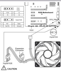
Connecting a strip to an incorrect connector can potentially cause damage to the LED strip, due to the RGB, and Digital RGB connectors providing different voltages .
